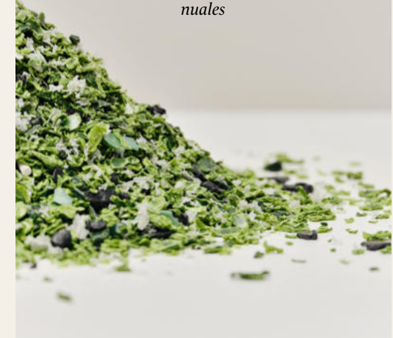
Plastic beer kegs Empty beer kegs are crushed and made into ready-to-use plastic gra- nuals
