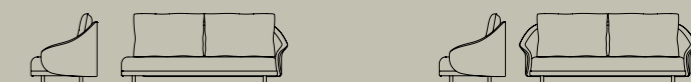
New Wave Sofa, Open-End W/D/H 211, 90, 94 CM SEAT HEIGHT 41 CM New Wave Sofa, Two-Seater W/D/H 224, 90, 94 CM SEAT HEIGHT 46 CM
